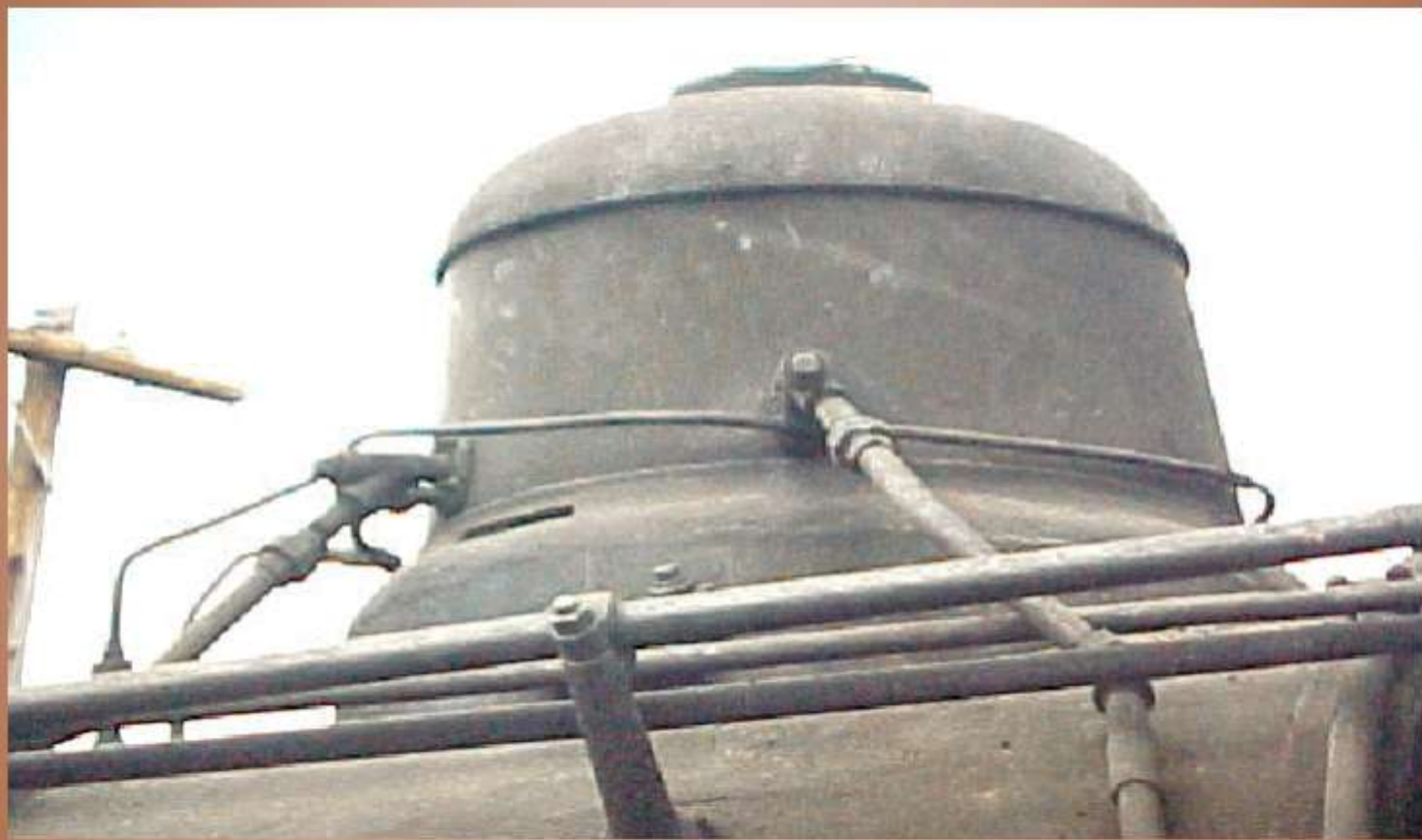
Piping Around Sand Dome on Current C&TT 497 Photo by Tony Kassin
