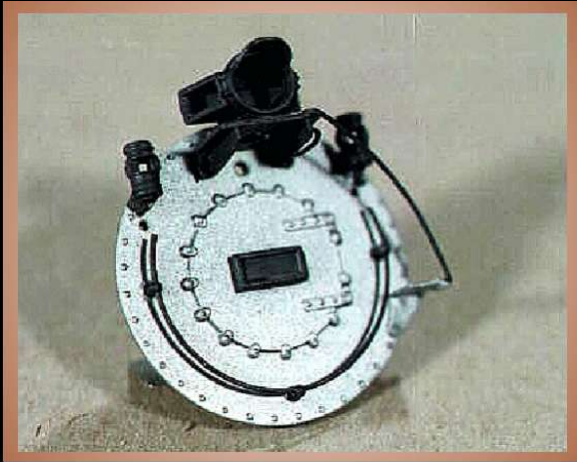
Air Brush Painted Boiler Face Plate Brush Painted Number Plate, Markers & Headlight
